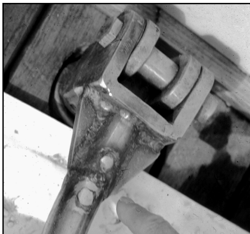
The tiller after repairs made by British Navy personnel at Port Stanley in the Falkland Islands. The point of the break necessitated inside sleeves installed and drilled at sea.
