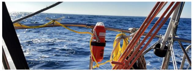
Gaskets from Brands that held the stays to the mast when taken down reused to hold the man overboard system.
