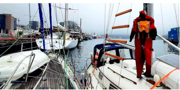
Drying out the immersion suit after getting into the freezing water to check the self steering servo pendulum.
