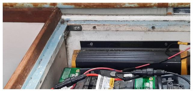
Used the vise to bend an angle to reseat the battery box.
