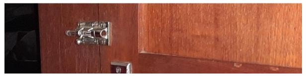
Head lock broke so installed a closure from the nav table.
