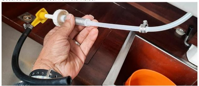
Extra epoxy pump for transferring alcohol to the stove from gallon cans. Used only 2-1/2 gallons
