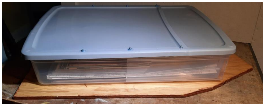
Chart box made from cutting an under the bed box, bolting them together.
